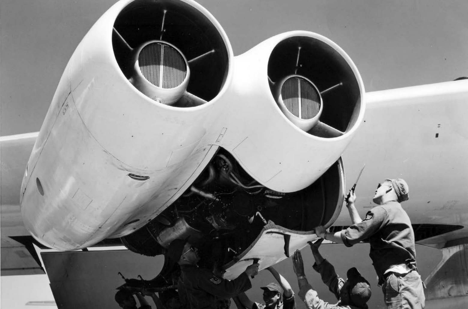
Airmen fix the cover on a BUFF's J57 jet engine at Offutt AFB, Neb., in the late 1950s. The Pratt & Whitney power plant was the first engine installed on the venerable bomber. The TF-33 equipped later models starting in 1961.
